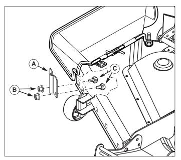
Figure 5. Install Mounting Plate
